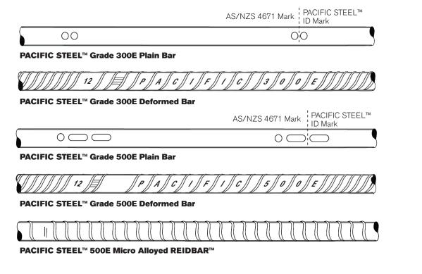
**IMPORTANT NOTE:** In line with our reinforcing brand update to PACIFIC STEEL<sup>™</sup>, the historical 'SEISMIC'® bar marking updated to 'PACIFIC<sup>™</sup> from June 2024. SEISMIC® continues to be a registered trademark of Pacific Steel (NZ) Ltd, and 300E/500E products featuring the former bar marking may still be observed in the market during this transition and treated as compliant.
